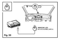
Install the status LED on the edge of the car's windshield. It must be convenient for entering a possible emergency **OVERRIDE CODE** using the button on its front, and at the same time visible both from inside the vehicle and outside. The LED informs you about the status of the alarm system (see the following table).
