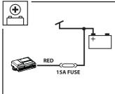
Connect the **POSITIVE SUPPLY +30** by placing a 15A fuse or if possible connecting on a protected line of the car.
